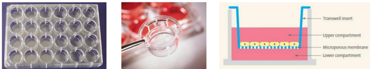
Figure 2-7: Transwell® Inserts Cell Culture Device. Cells were cultured on microporous membrane and ^{239}\text{Pu} colloids were deposited in the upper compartment. Activity measurements (liquid scintillation) were carried out on lower compartment media samples at different times post-contamination.
